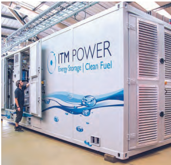
FIGURE 3.9 ITM PEM electrolyzer National Physics Lab, United Kingdom, 2019 (left) and Siemens Silyzer 3000, Mainz Park, Germany, 2019 (right)
