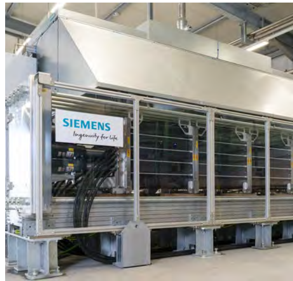
FIGURE 3.9 ITM PEM electrolyzer National Physics Lab, United Kingdom, 2019 (left) and Siemens Silyzer 3000, Mainz Park, Germany, 2019 (right)
