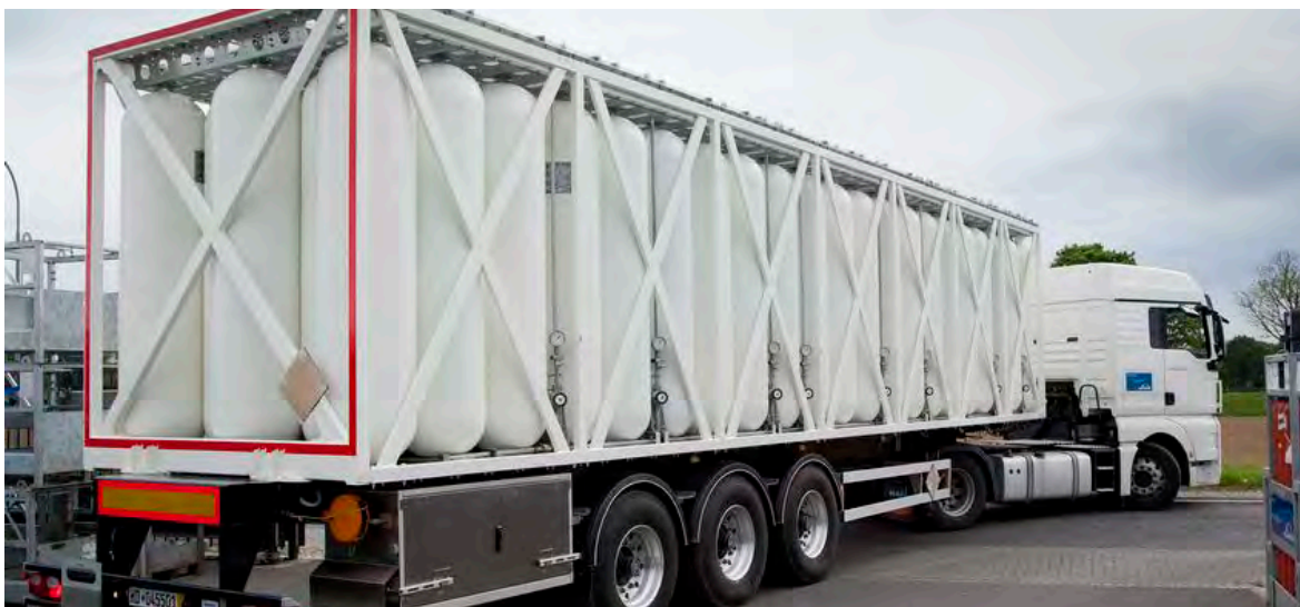
FIGURE 7.5 Pressurized hydrogen storage trailers
